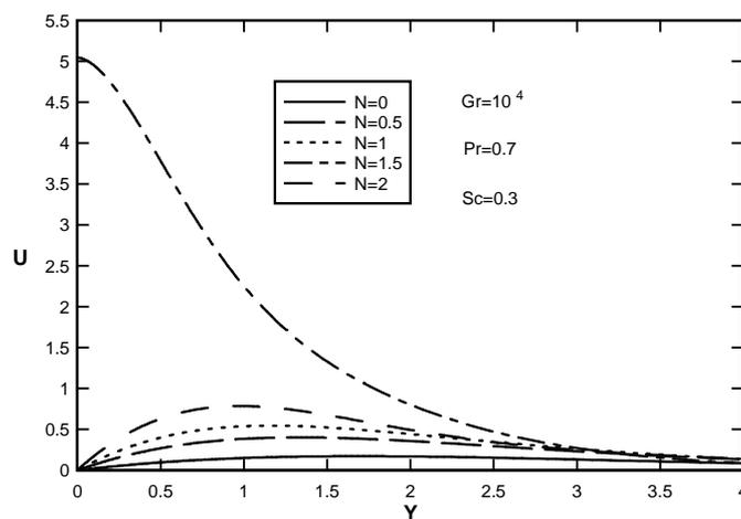
Figure 5. Effect of buoyancy ratio parameter ( $N$ ) on dimensionless velocity Profiles at dissipation number ( $\mathcal{E} = 1.0$ )
