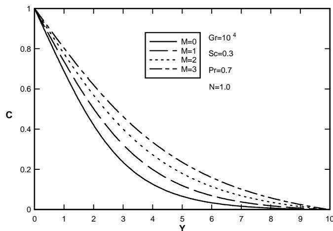
Figure 4. Effect of magnetic parameter on dimensionless concentration distributions dissipation number ( $\mathcal{E} = 1.0$ )
