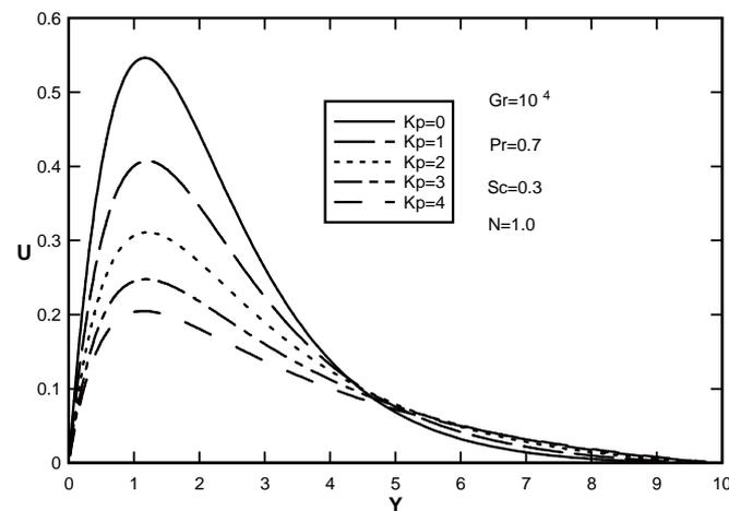
Figure 11. Effect of porous media parameter ( $K_p$ ) on dimensionless velocity Profiles at dissipation number ( $\mathcal{E} = 1.0$ )
