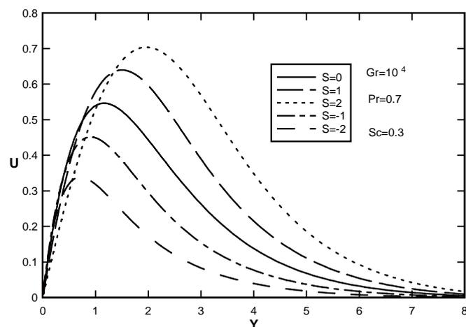
Figure 8. Effect of Suction rate parameter ( $S$ ) on dimensionless velocity Profiles at dissipation number ( $\mathcal{E} = 1.0$ )
