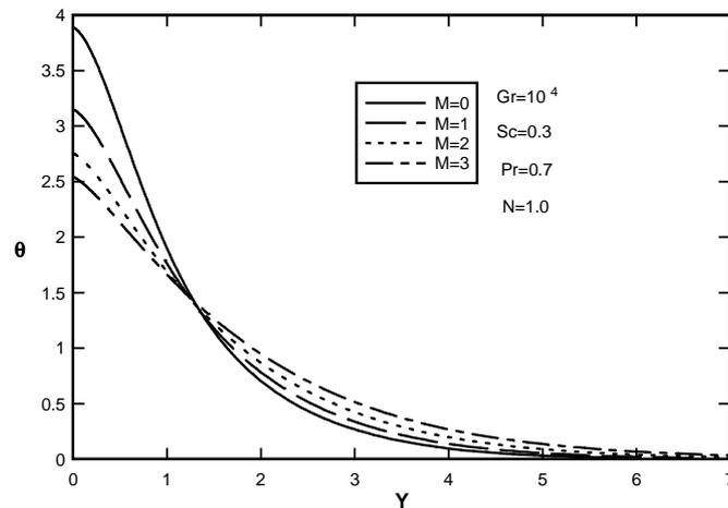
Figure 3. Effect of magnetic parameter on dimensionless temperature distributions at dissipation number ( $\mathcal{E} = 1.0$ )
