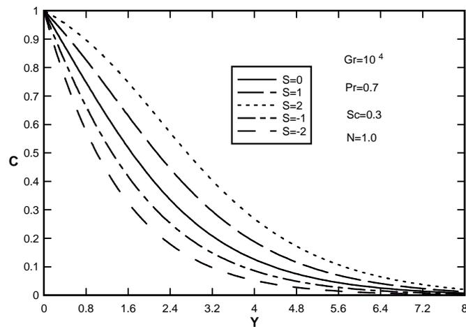
Figure 10. Effect of Suction rate parameter ( $S$ ) on dimensionless concentration distributions dissipation number ( $\mathcal{E} = 1.0$ )
