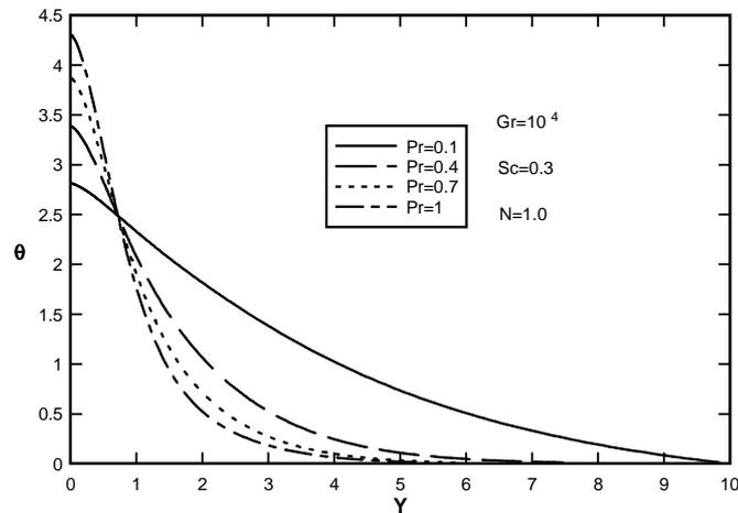
Figure 15. Effect of Prandtl number (Pr) on dimensionless temperature distributions at dissipation number ( $\mathcal{E} = 1.0$ )
