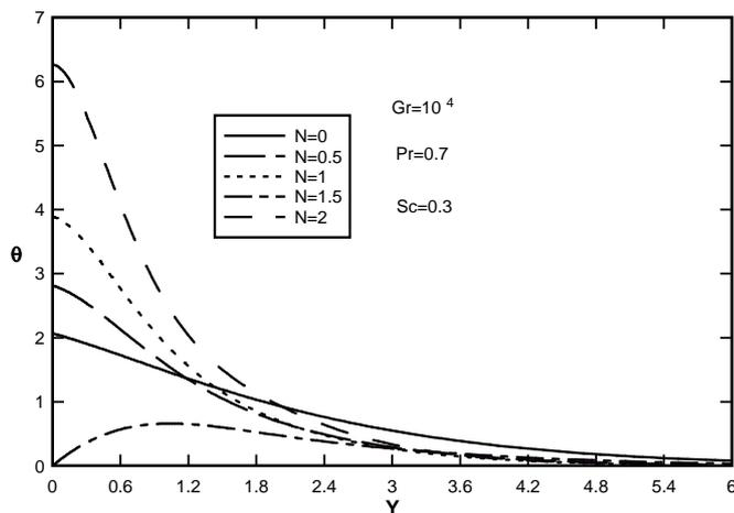
Figure 6. Effect of buoyancy ratio parameter (N) on dimensionless temperature distributions at dissipation number ( $\mathcal{E} = 1.0$ )
