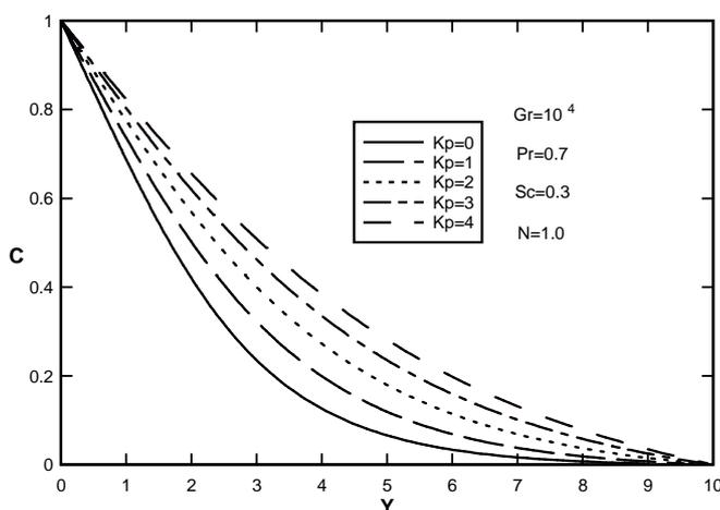
Figure 13. Effect of porous media parameter ( $K_p$ ) on dimensionless concentration distributions dissipation number ( $\mathcal{E} = 1.0$ )
