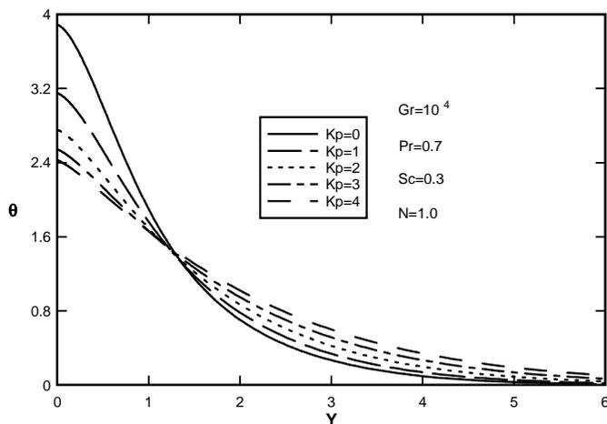
Figure 12. Effect of porous media parameter ( $K_p$ ) on dimensionless temperature distributions at dissipation number ( $\mathcal{E} = 1.0$ )
