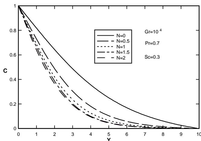
Figure 7. Effect of buoyancy ratio parameter (N) on dimensionless concentration distributions dissipation number ( $\mathcal{E} = 1.0$ )
