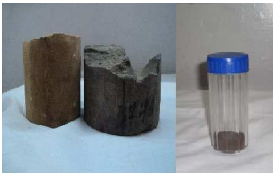
Figure-1. Two cylindrical samples of oil-well core were taken from the drillers and the sample container for irradiate the detectors.
