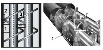
Figure 2 Shear zones in TS-LTE: Screw channel gap (zone 1), clearance gap (zone 2), tangential gap (zone 3) and screw roots gap (zone 4).
