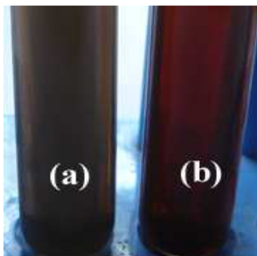
Fig.1. colour change yellow to brown indicate formation silver nanoparticles (a) leaf extract (b) after addition of leaf extract into 1 mM \text{AgNO}_3
