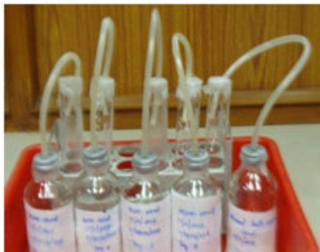
Figure 3: Experimental setup for mineralization of latex.
