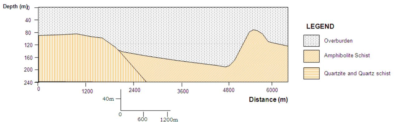
Figure 3a Geomagnetic Section along Traverse 11 (SE - NW) of the study area Area
