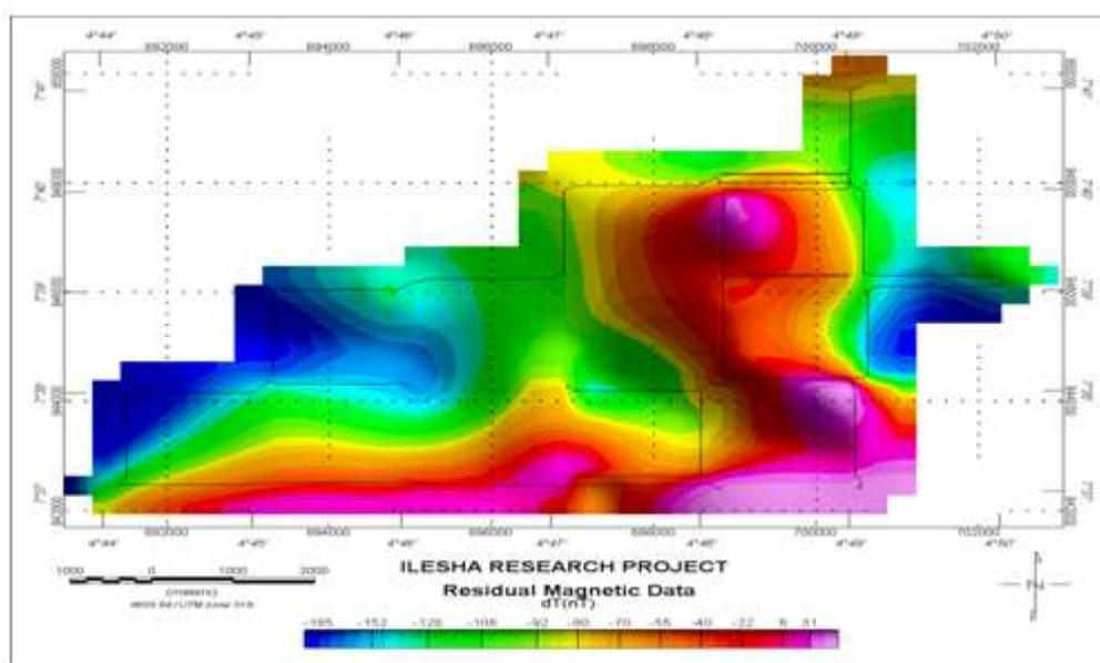
Figure 4: Residual magnetic map of the study area using Total Relative Magnetic Intensity.
