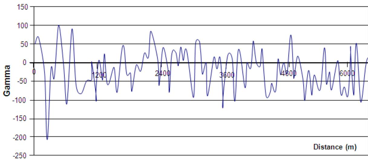
Figure 2a Total Relative Magnetic Intensity along Traverse 11 (SE - NW) of the study area
