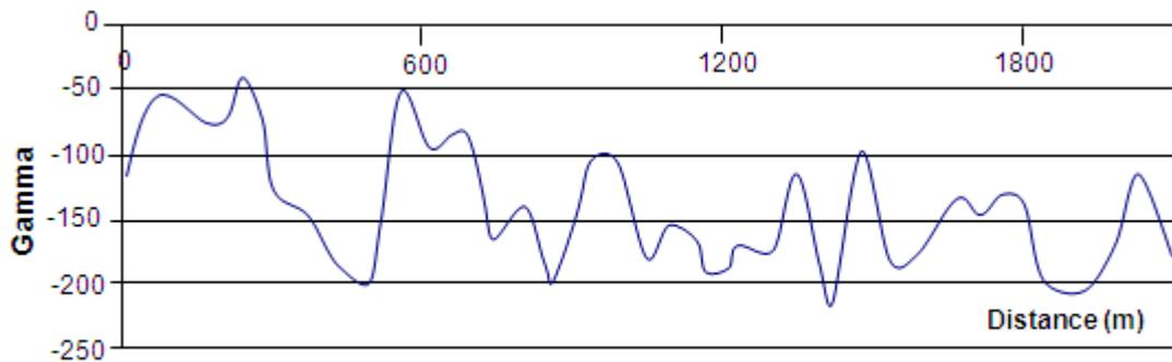
Figure 2d Total Relative Magnetic Intensity along Traverse 15 (NW - SE) of the study area
