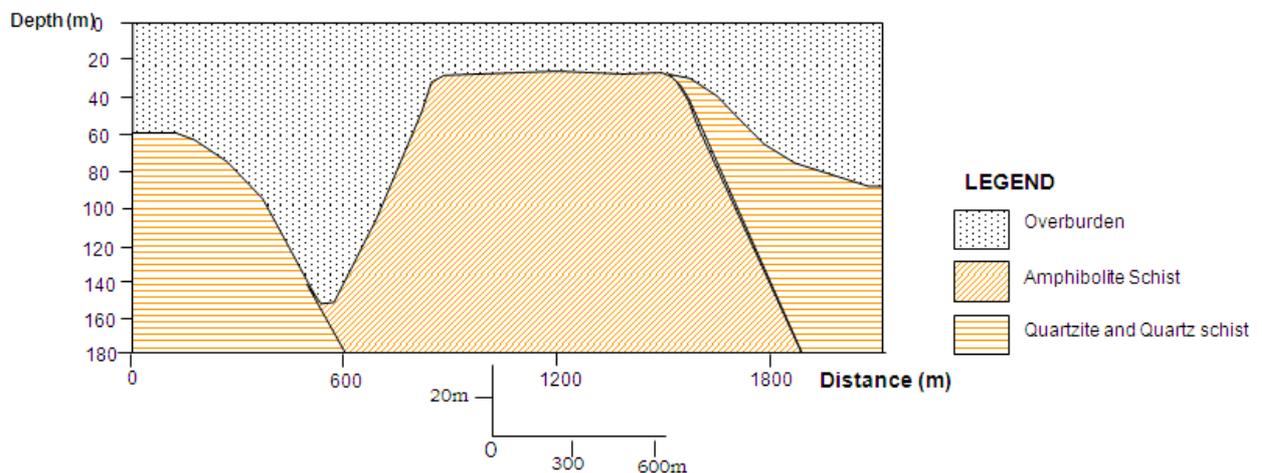
Figure 3d Geomagnetic Section along Traverse 15 (NW - SE) of the study area
