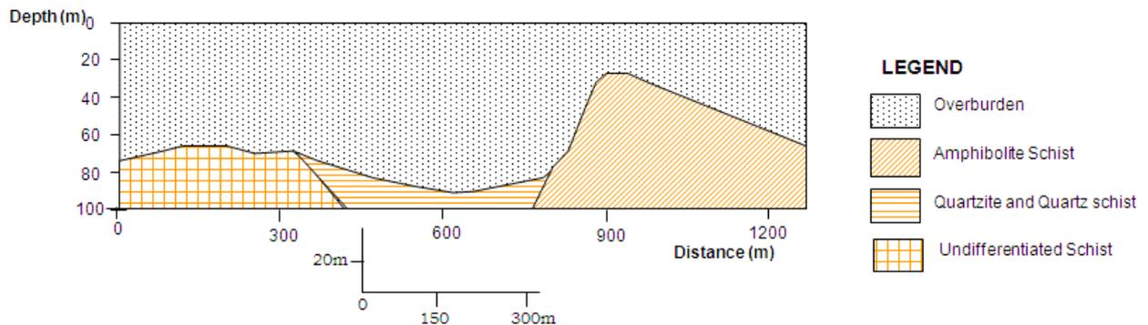
Figure 3c Geomagnetic Section along Traverse 14 (SE - NW) of the study area
