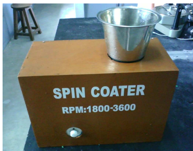
Fig. 1: Spin Coater with spill arrestor
