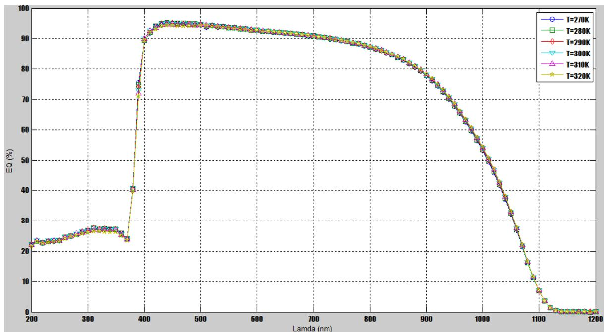
Fig. 5: Variation of external quantum efficiency according to the wavelength for various use temperatures of the Cu(In,Ga)Se<sub>2</sub> thin film solar cell
