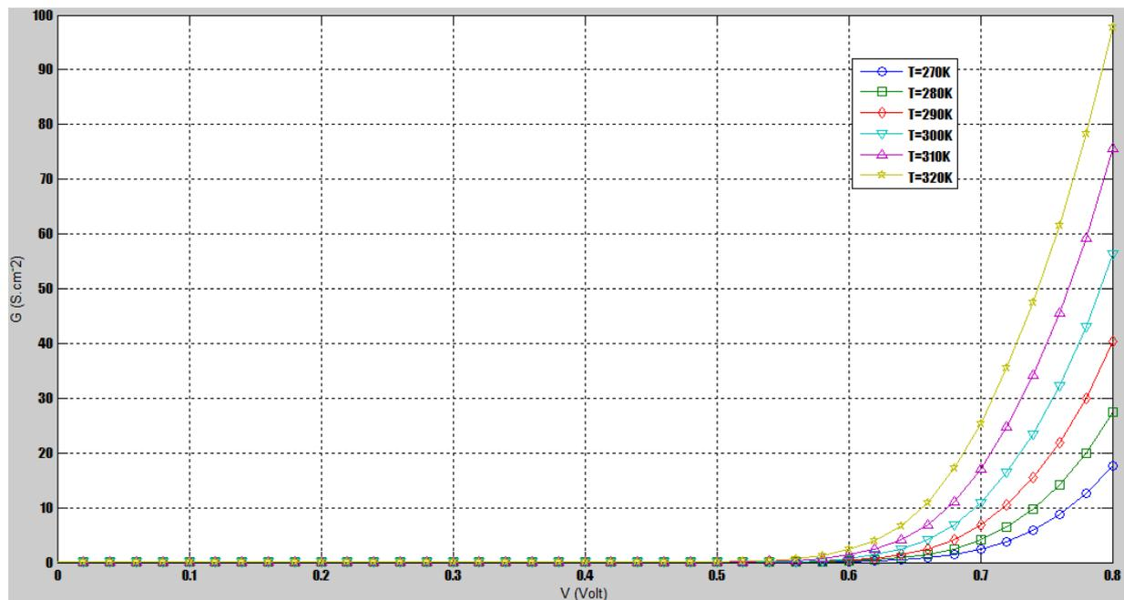
Fig. 4: Variation of the generation of the minority carriers according to the tension for various temperatures of use
