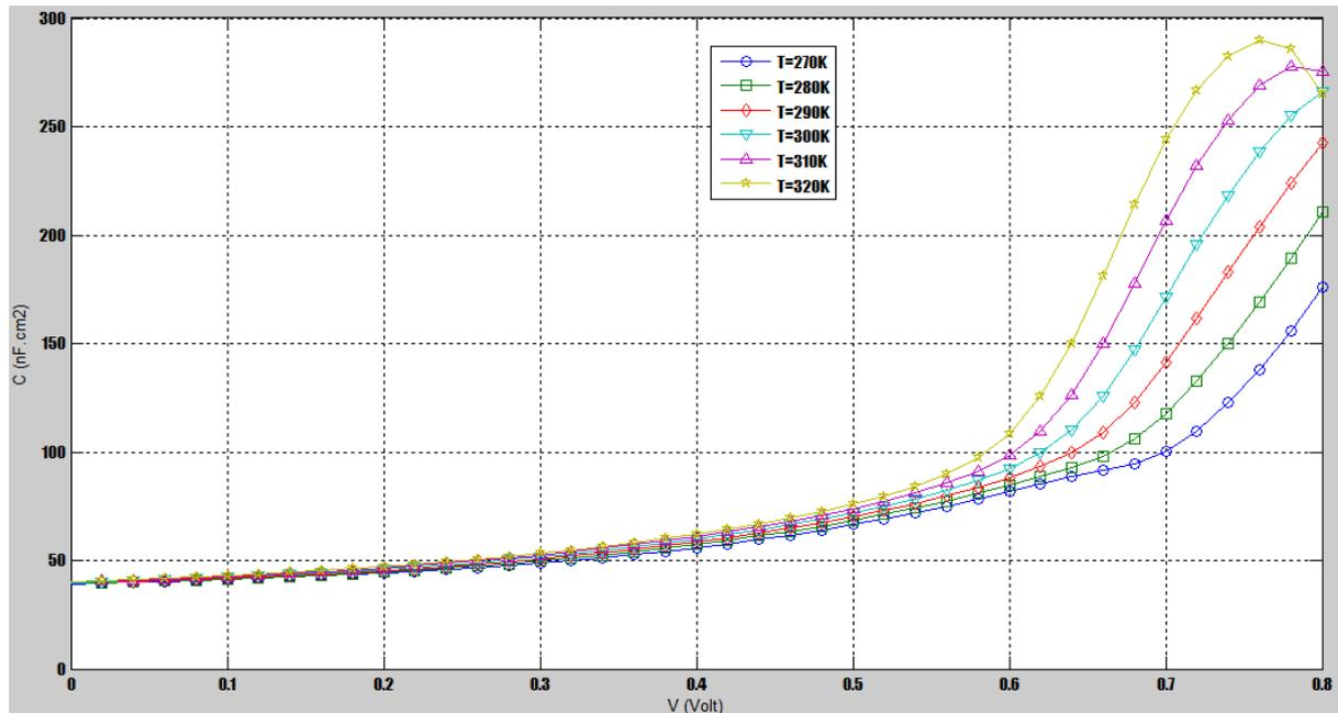
Figure 2: Variation of the capacitance according to the voltage for various use temperatures of the Cu(In,Ga)Se<sub>2</sub> thin film solar cell
