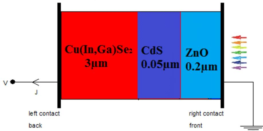
Fig. 1: The Cu(In,Ga)Se<sub>2</sub> thin film solar cell configuration
