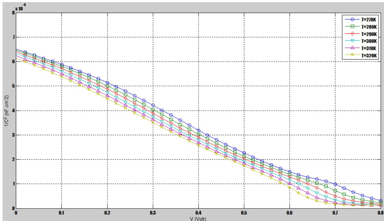
Fig. 3: Variation of the reverse of the square of the capacitance according to the voltage for various use temperatures of the Cu(In,Ga)Se<sub>2</sub> thin film solar cell
