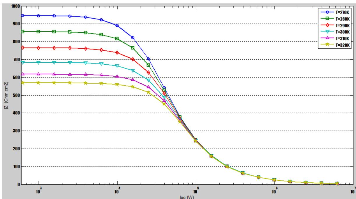
Fig. 6: The variation of the module of the impedance according to the logarithm of the pulse for various use temperatures of the Cu(In, Ga)Se<sub>2</sub> thin film solar cell
