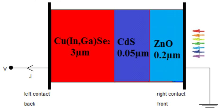
**Fig. 1: The configuration of the Cu(In, Ga)Se<sub>2</sub> thin film solar cell studied**
