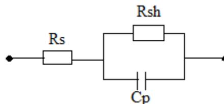
Fig. 4: The equivalent circuit of the capacitive effects of the studied solar cell
