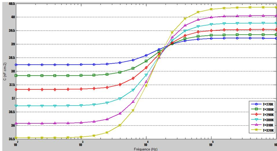
Fig. 2: The variations of the capacitance according to the frequency for various use temperatures of the Cu(In,Ga)Se<sub>2</sub> thin film solar cell
