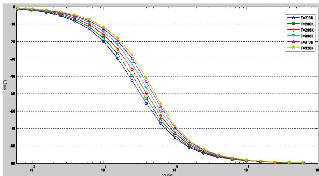
Fig. 3: The variation of the phase  $\Phi$  of the impedance according to the logarithm of the impulse for various use temperatures of the Cu(In, Ga)Se<sub>2</sub> thin film solar cell
