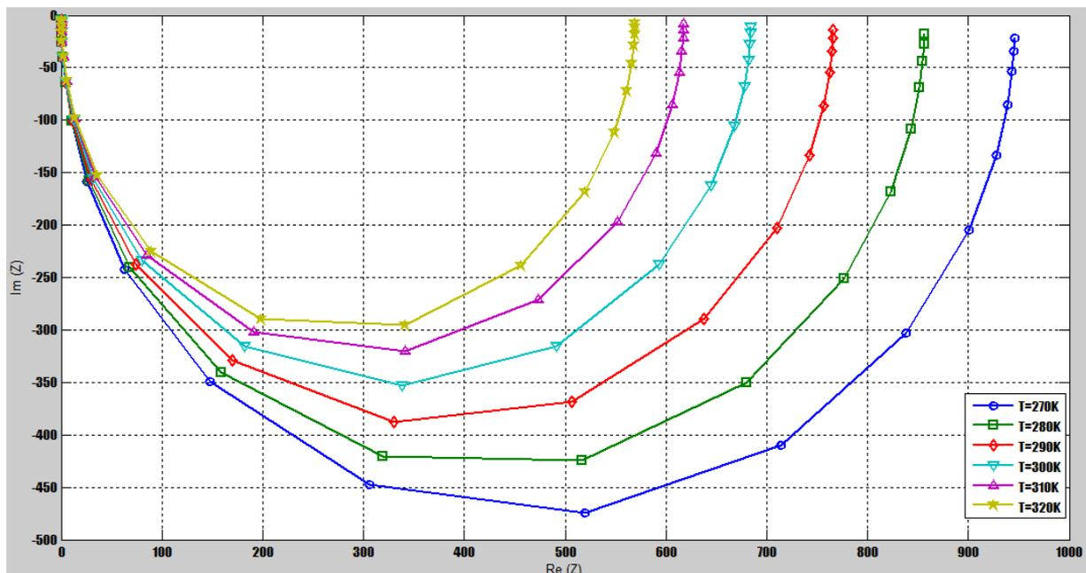
Fig. 5: The Nyquist plots of the Cu(In,Ga)Se<sub>2</sub> thin film solar cell for various use temperatures
