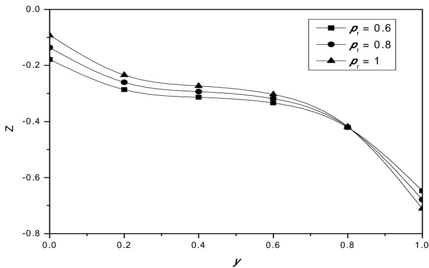
Figure 14- Effect of  $P_r$  on variation of  $Z$  for  $d = 0.1, b = 0.1, \theta = \pi/3, a = 0.1, \delta = 0.01, R = 1, E_1 = 0.1, E_2 = 0.2, E_3 = 0.3, E = 1$
