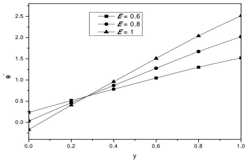
Figure 7-Effect of  $E$  on variation of  $\theta^*$  for  $d = 0.1, b = 0.1, \theta = \pi/3, a = 0.1, \delta = 0.01, R = 1, E_1 = 0.1, E_2 = 0.2, E_3 = 0.3, P_r = 0.7$
