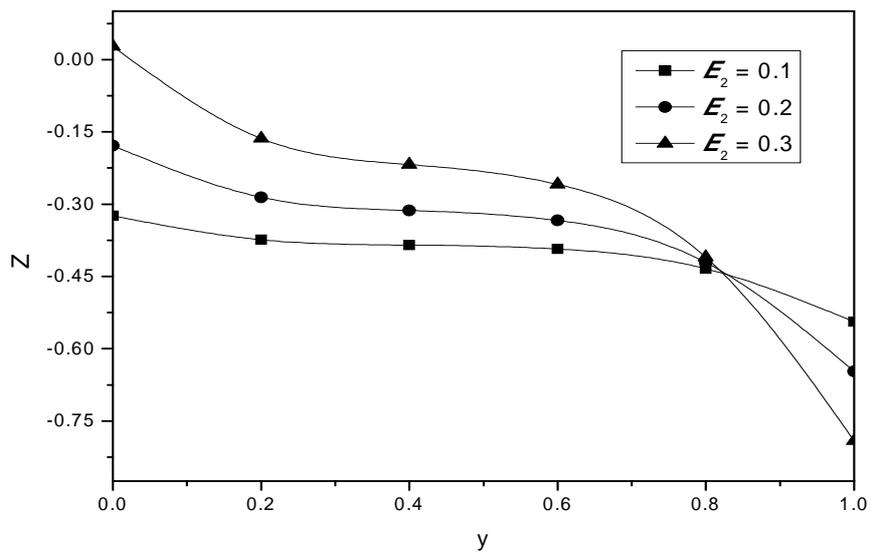
Figure 11- Effect of  $E_2$  on variation of  $Z$  for  $d = 0.1, b = 0.1, \theta = \pi/3, a = 0.1, \delta = 0.01, R = 1, E_1 = 0.1, E_3 = 0.3, E = 1, P_r = 0.7$
