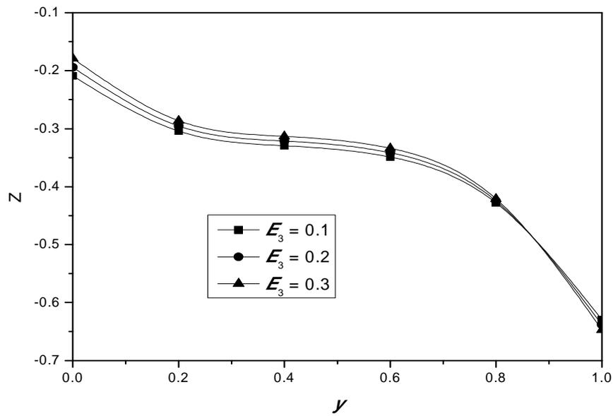
Figure 12- Effect of  $E_3$  on variation of  $Z$  for  $d = 0.1, b = 0.1, \theta = \pi/3, a = 0.1, \delta = 0.01, R = 1, E_1 = 0.1, E_2 = 0.2, E = 1, P_r = 0.7$
