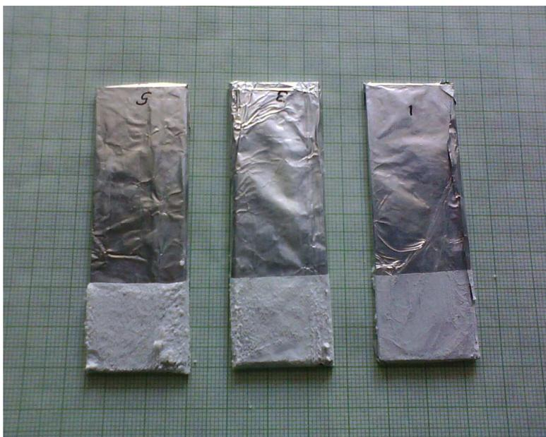
**Fig.1: Electrodeposited ZnO on Aluminum foil**
