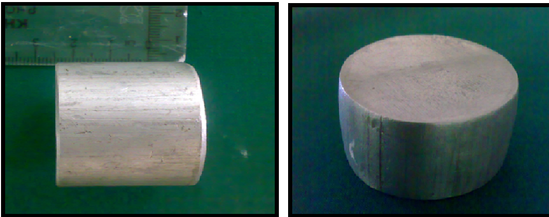
(a) (b) Figure 9 (a) Aluminum billet of size height 40 mm dia.40 mm before compression (b) Aluminum billet of size height 40 mm dia.40 mm after compression
