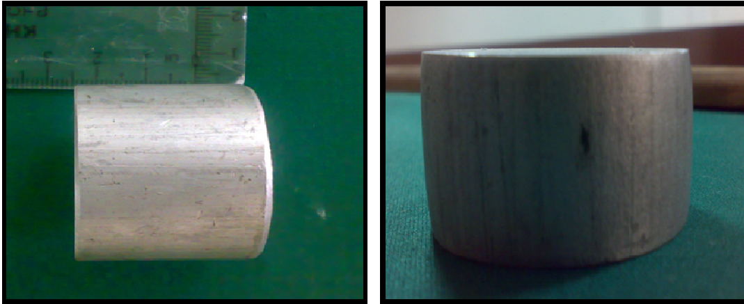
(a) (b) Figure 8 (a) Aluminium billet of height 30 mm diameter 40 mm before compression (b) Aluminium billet of height 30 mm diameter 40 mm after compression
