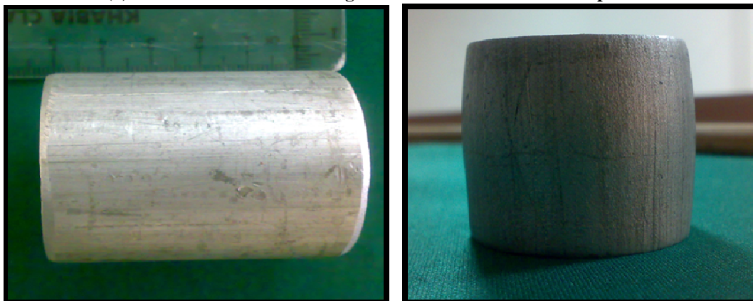
(a) (b) Figure 10 (a) Aluminium billet of height 50 mm diameter 40 mm before compression (b) Aluminium billet of height 50 mm diameter 40 mm after compression
