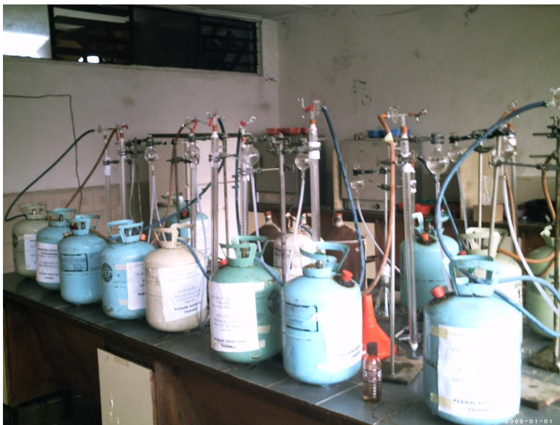
PLATE 3: Experimental Set-up showing the different weights of cow dung used for biogas generation
