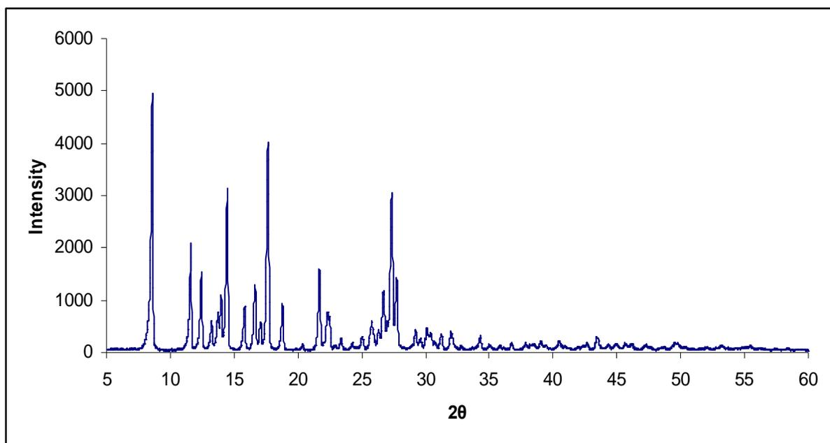
Figure. 13(A): X-ray diffraction pattern of pure GBM
