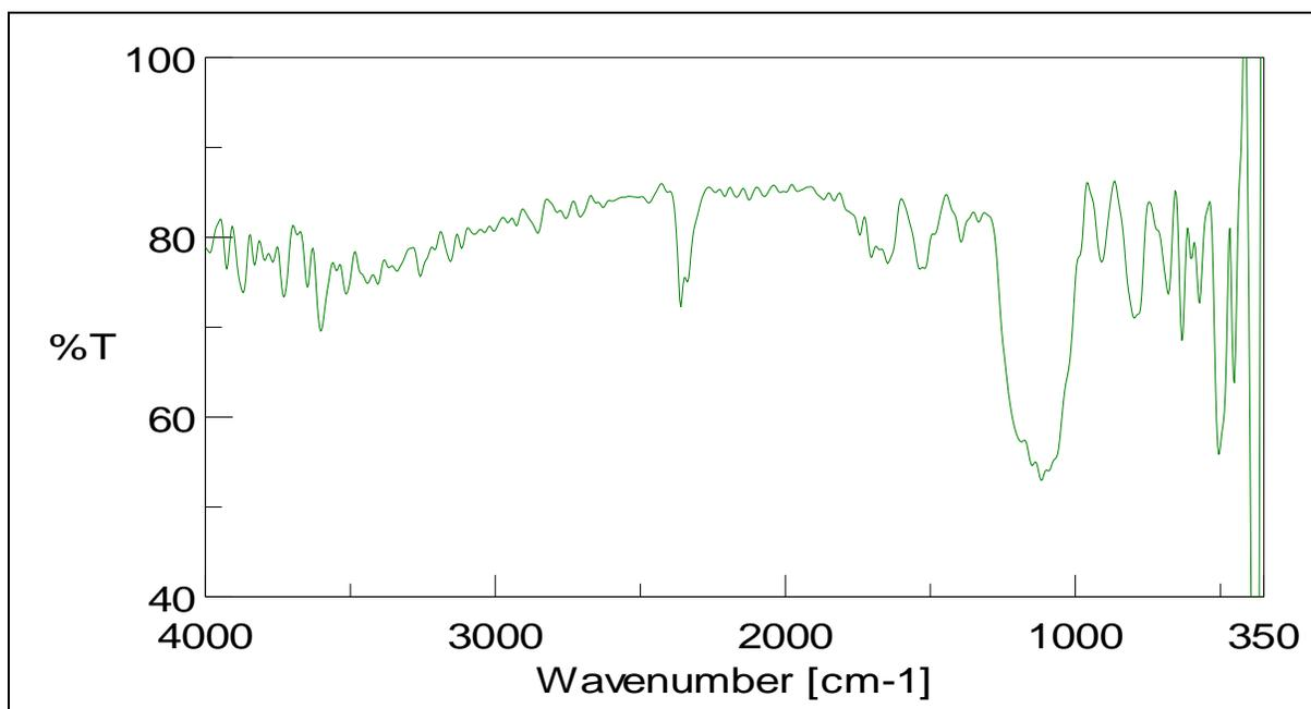
Figure. 12(B): Infrared spectrum of Aerosil 200
