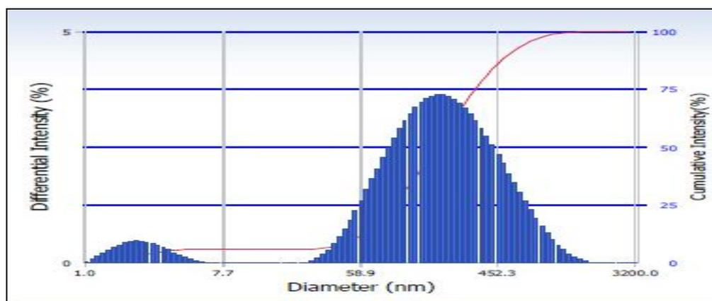
Figure.8. Droplet size of optimized Solid SEDDS batch (S-1)
