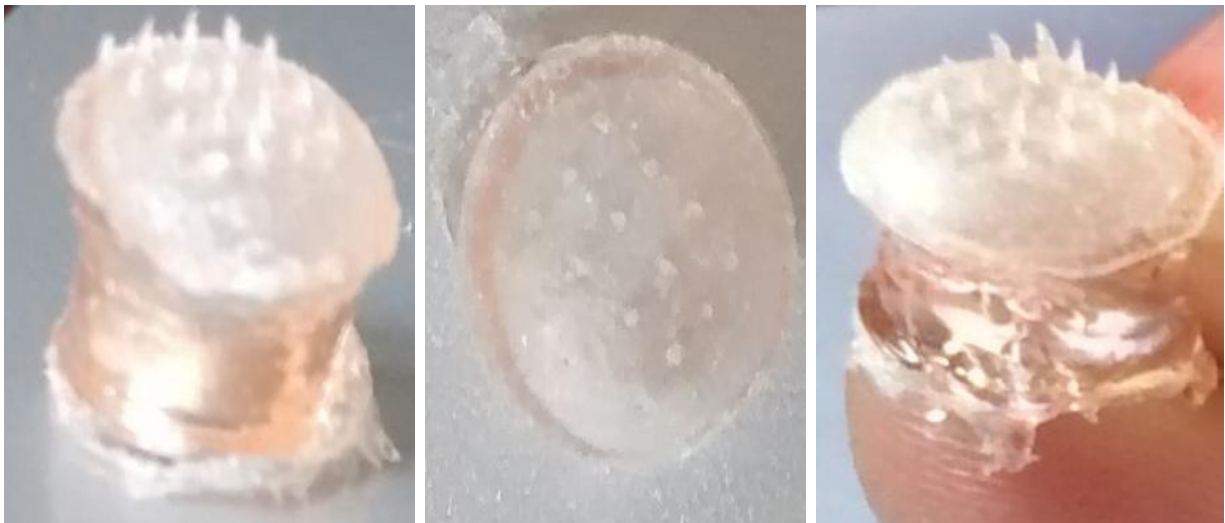
Figure 3. Micro needle array patches with sharp tips and uniform assembly
