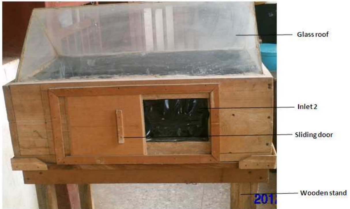
Figure 3. Direct Absorption Solar Dryer (DASD) showing the sliding door
