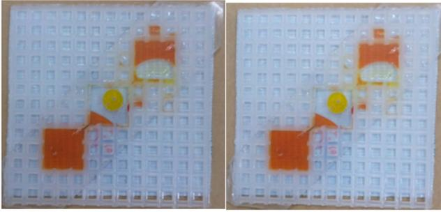
**Figure 8:** Size of canvas reduced to one passage. Fluid remained for a small period of time.
