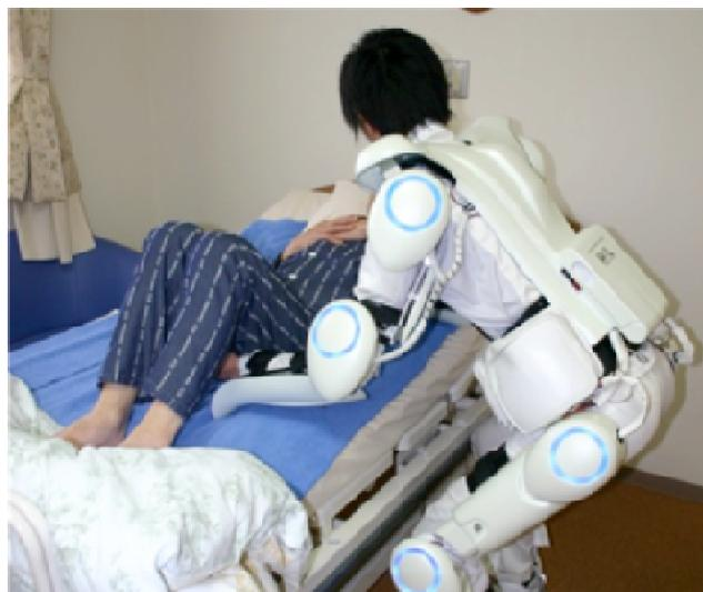
**Figure 1 : Example setting of the HAL-5 robot suit for nursing care.**
