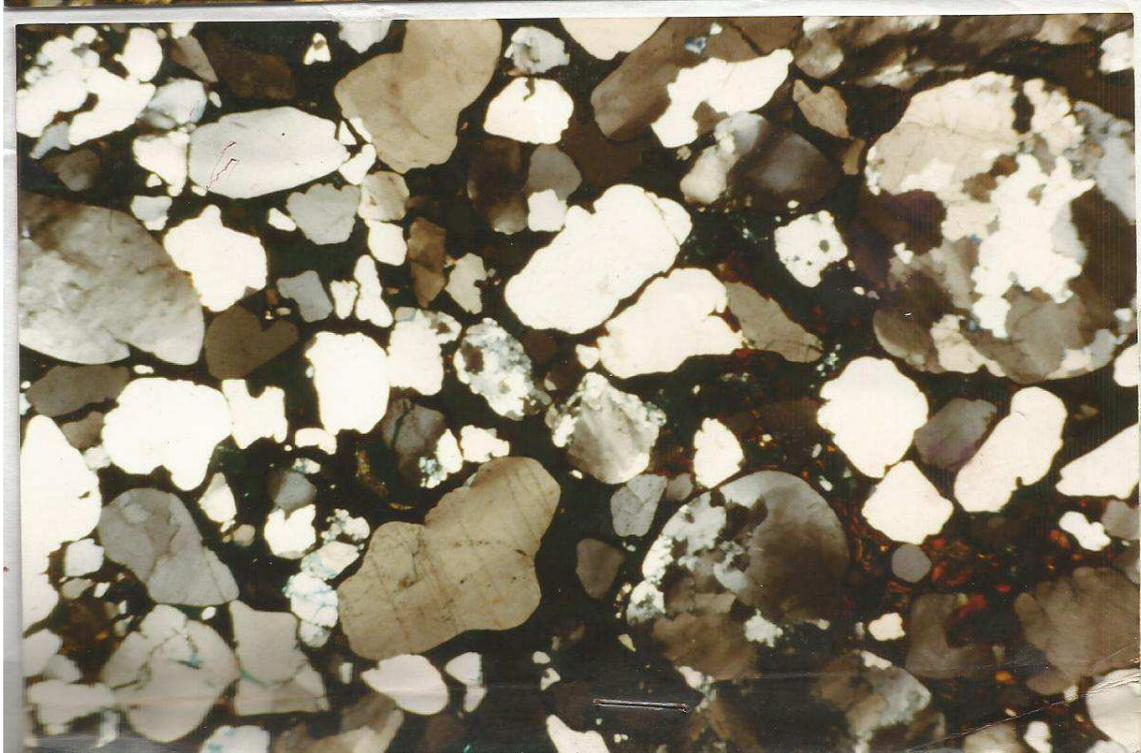
Fig.8. Thin-section photomicrograph of porous and permeable sandstone associated with hydrocarbon stains Detrital Mineralogy
