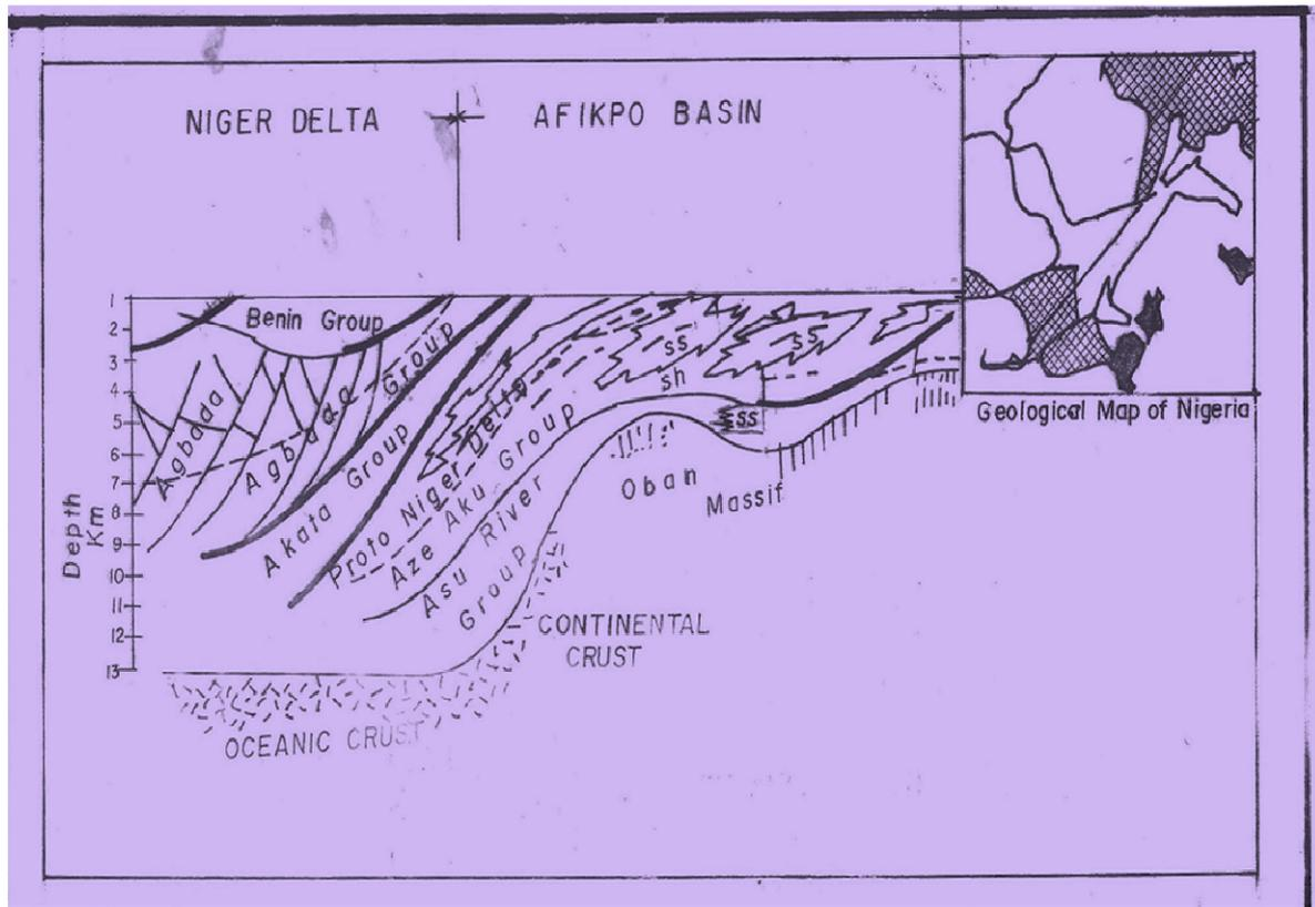
Figure 1: Synthetic Cross Section from the Niger Delta to Afikpo Basin Showing the Relationships between the various Lithostratigraphic units. The basement depth is obtained from the geophysical data
