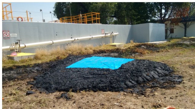
Figure 6: Start to the method of static stack of maturation, with the plastic cover for protection of the outdoor or open sky.
