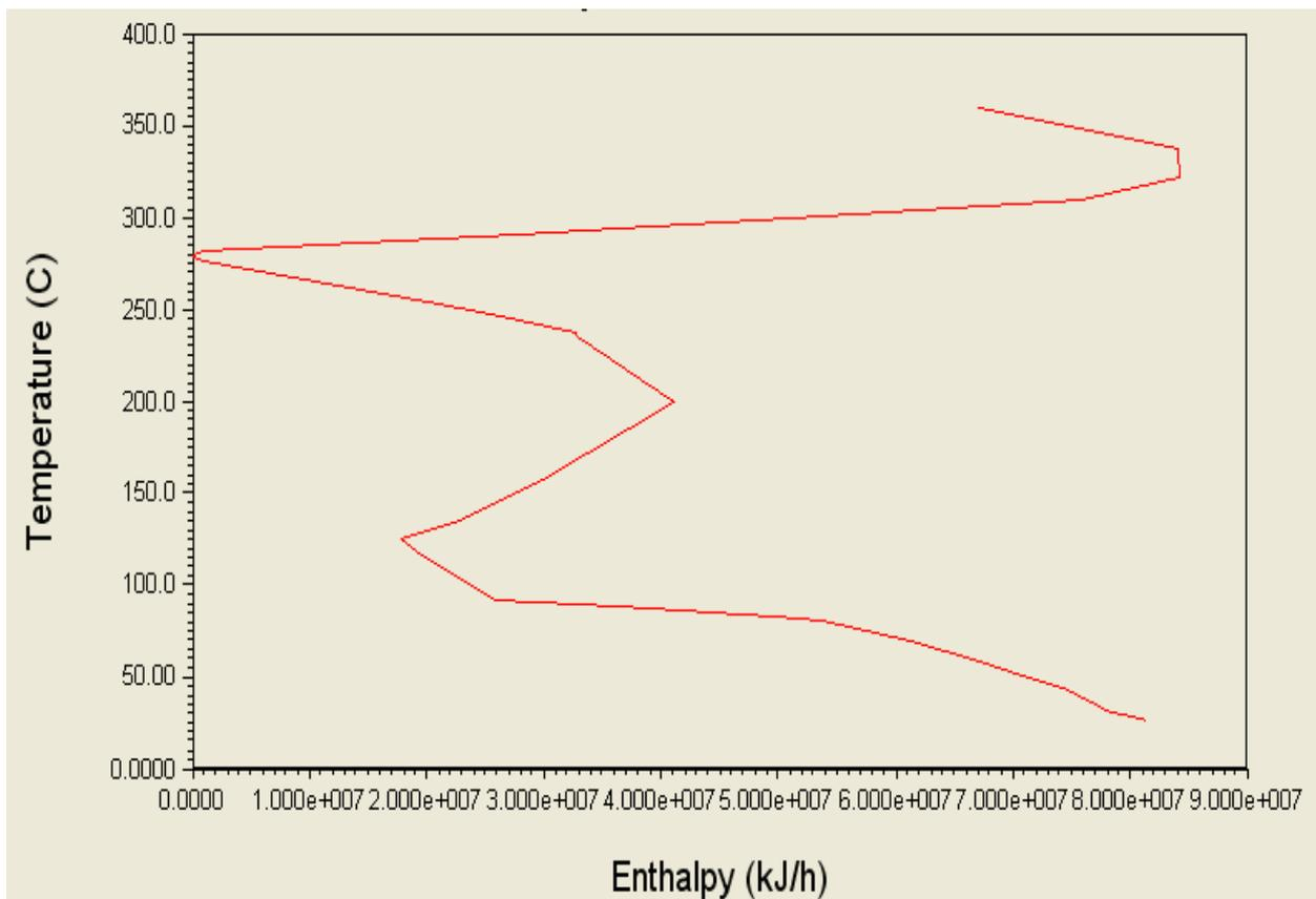
**Figure 5 Grand Composite Curve of Catalytic Reforming Unit**
