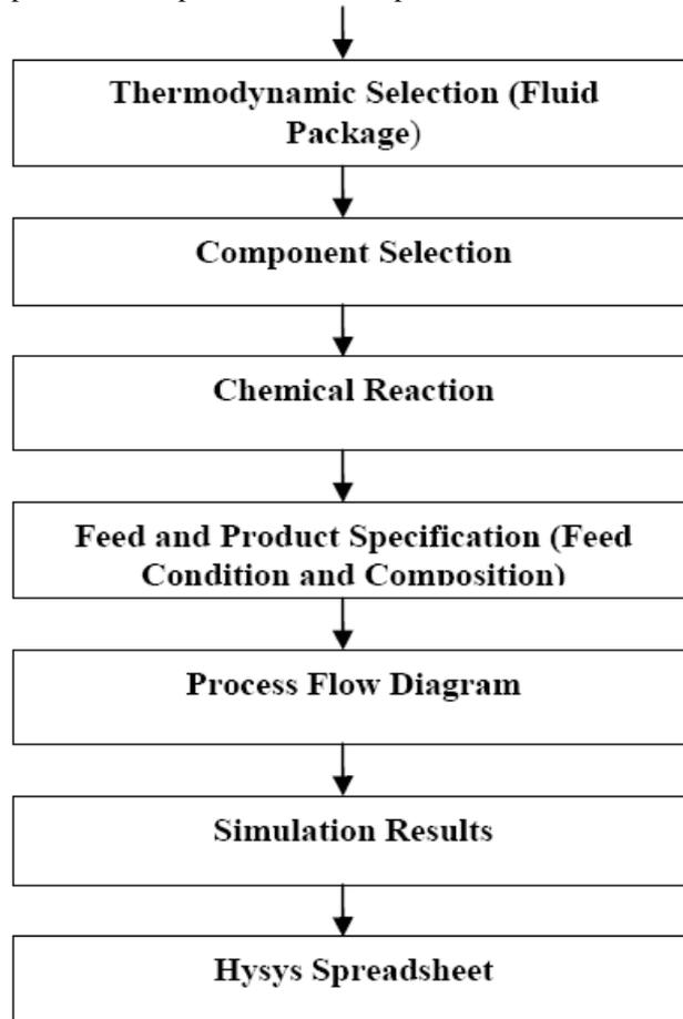
**Figure 2: Process Simulation Steps using HYSYS**
