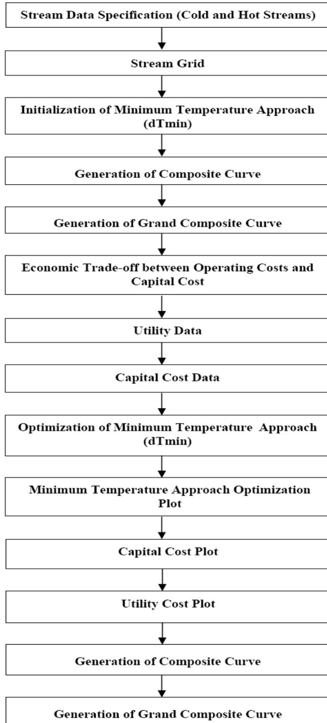
**Figure 3: Pinch Analysis Simulation Procedure**
