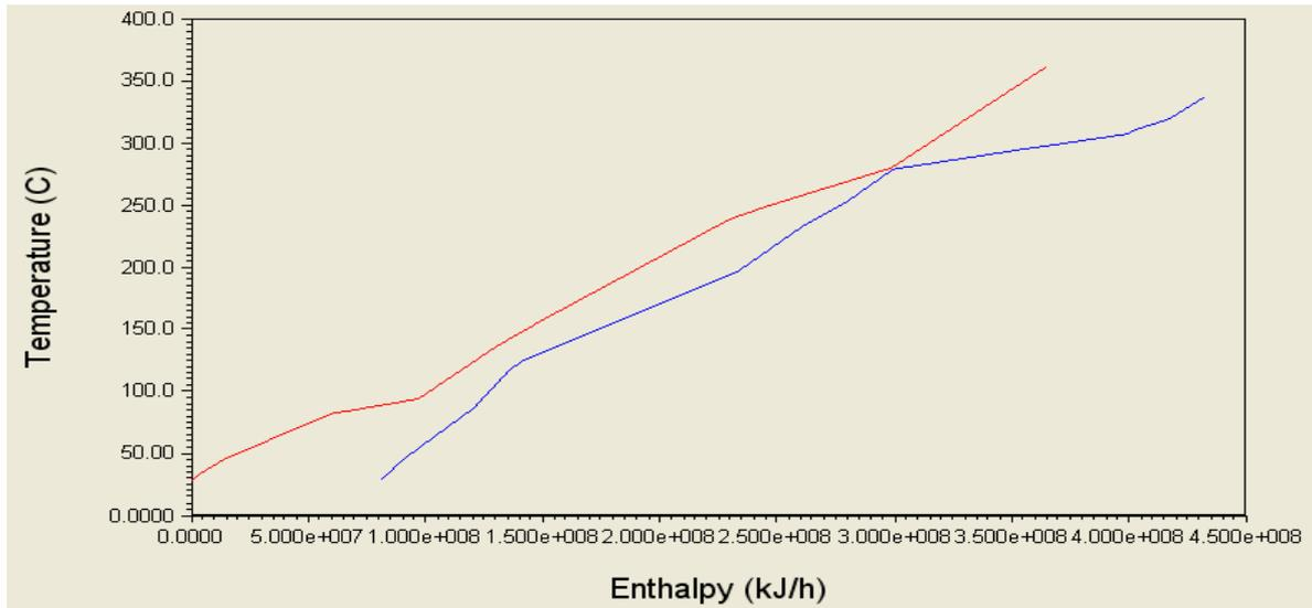
**Figure 4 Shifted Composite Curve of Catalytic Reforming Unit**
