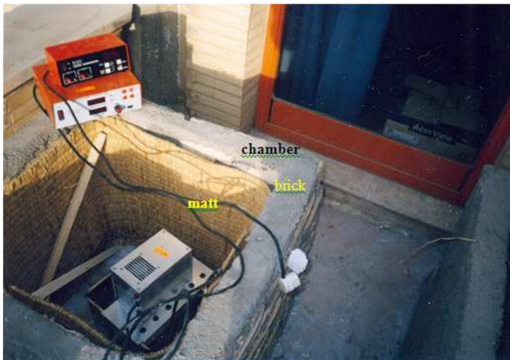
Fig.5 Brick chamber with the mat
