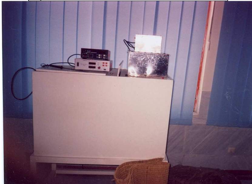
Fig2.The insulation chamber and temperature controller
