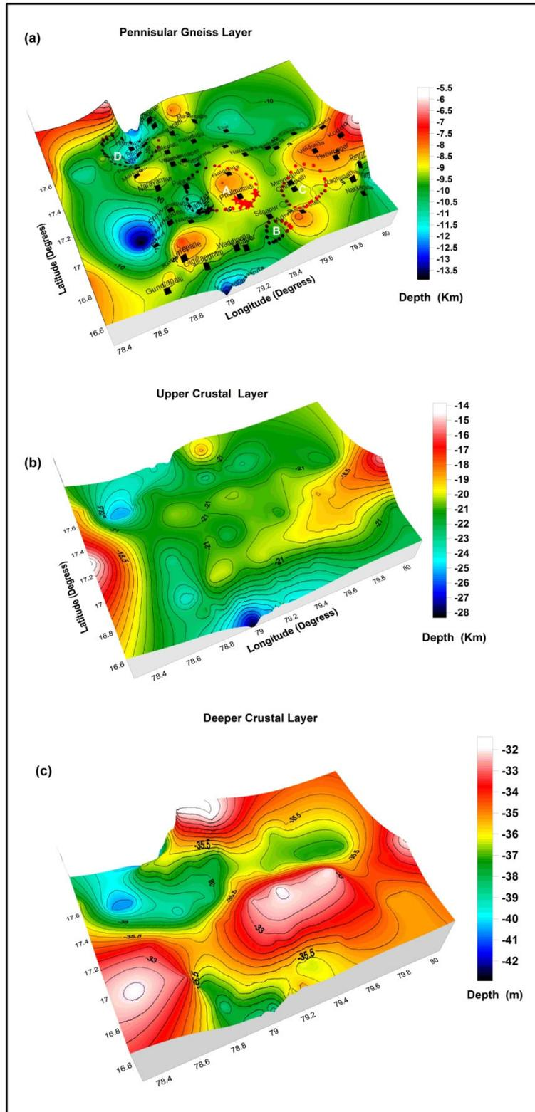
Figure 4.(a) 3D view of the Peninsular Gneissic layer (with density of 2.67 gm/cc) (b) 3D view of the Upper crustal layer (with density of 2.72 gm/cc) and (c) 3D view of the deeper crustal layer (with density of 2.85gm/cc) of Nalgonda district, Telangana
