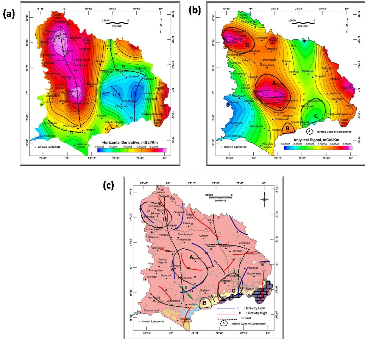
Figure 2. (a) Horizontal derivative map (X direction) of the Nalgonda district, Telangana (shows location of inferred gravity faults (F1 to F7)), (b) Analytical Signal map of the Nalgonda district, Telangana (shows locations of known Lamproites and three circular clusters A, B, C & D), (c) Integrated structural map of Nalgonda district, Telangana from the gravity qualitative analysis superimposed on Geology
