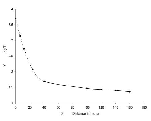
Fig 3 Temperature vs distance curve in Dikom fire
