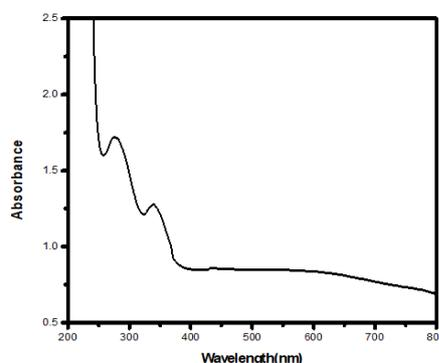
Figure 2: UV spectrum of Ag-NPs and Ag-MgO NCs.
