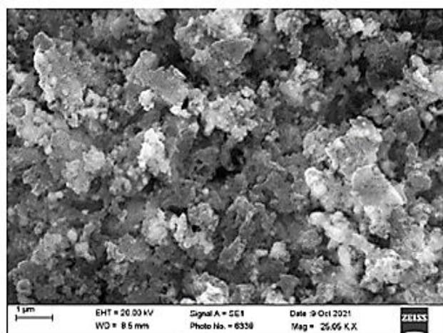
**Figure 4:** SEM micro images of fabricated Ag-MgO NCs.
