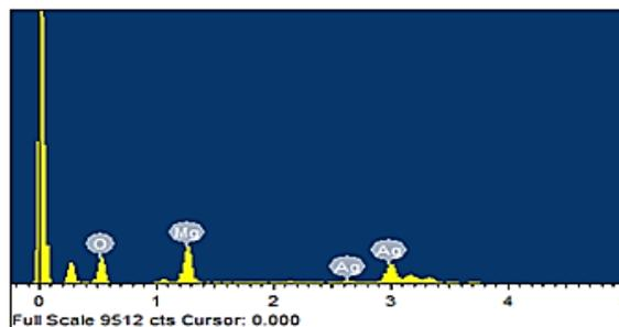
**Figure 5:** SEM-EDX data of synthesized Ag-MgO NCs.
