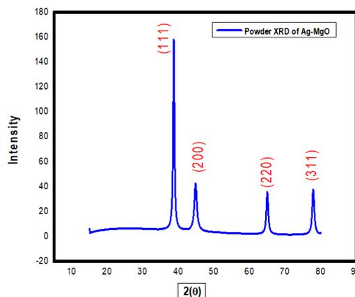
Figure 3: XRD of fabricated Ag-MgO NCs.
