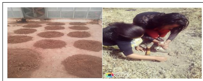
(a) Soils sample on air drier house (b) Soil sample for measuring bulk density
