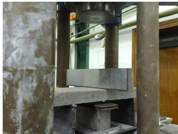
Figure 3. Set up for three point bending test
