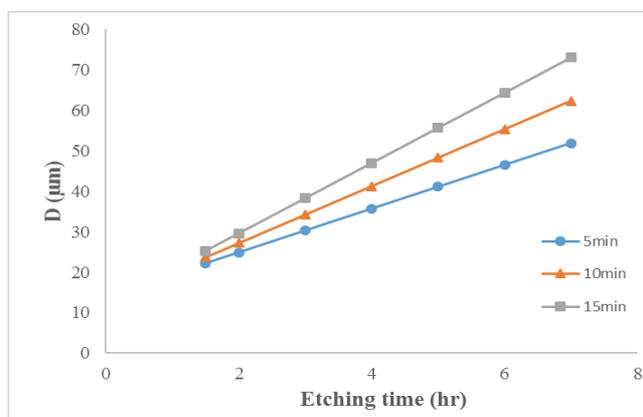
Figure 1: Alpha tracks diameter vs. etching time exposed to He-Ne laser beam at (1 mW) power etched in 6.25 N NaOH at  $60^\circ\text{C}$
