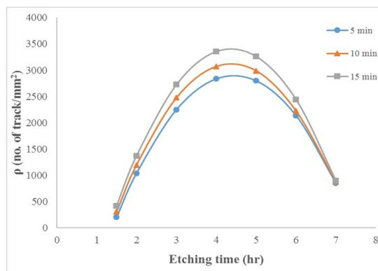
**Figure 5:** Alpha tracks densities vs. etching time exposed to He-Ne laser beam at power (5 mW) at different times etched in 6.25 N NaOH at 60°C
