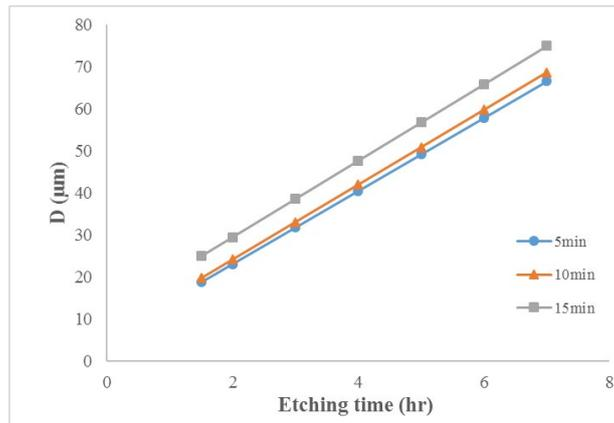
**Figure 3:** Alpha tracks diameter vs. etching time exposed to He-Ne laser beam at (10 mW) power etched in 6.25 N NaOH at 60°C
