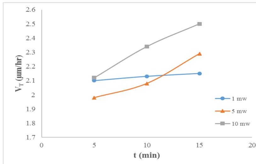
**Figure 12:** Track etch rate  $V_T$  vs. exposure time of He-Ne laser beam at different powers
