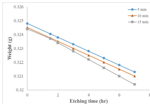
**Figure 8:** Weight of CR-39 detector vs. etching time at different exposed times to He-Ne laser beam at (5mW)
