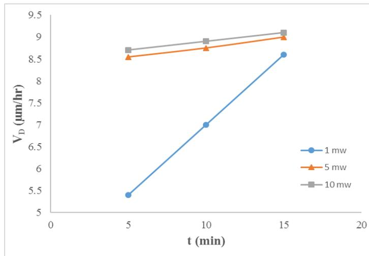
**Figure 10:** Diameter etch rate  $V_D$  vs. exposure time of He-Ne laser beam at different powers
