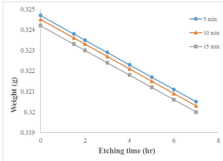
**Figure 9:** Weight of CR-39 detector vs. etching time at different exposed times to He-Ne laser beam at (10 mW)
