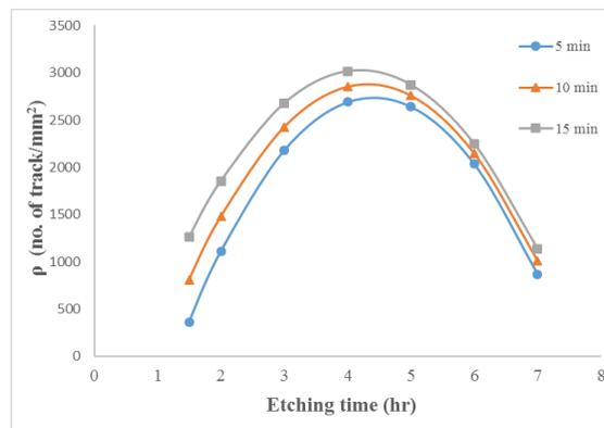
**Figure 4:** Alpha tracks densities vs. etching time exposed to He-Ne laser beam at power (1 mW) at different times etched in 6.25 N NaOH at 60°C
