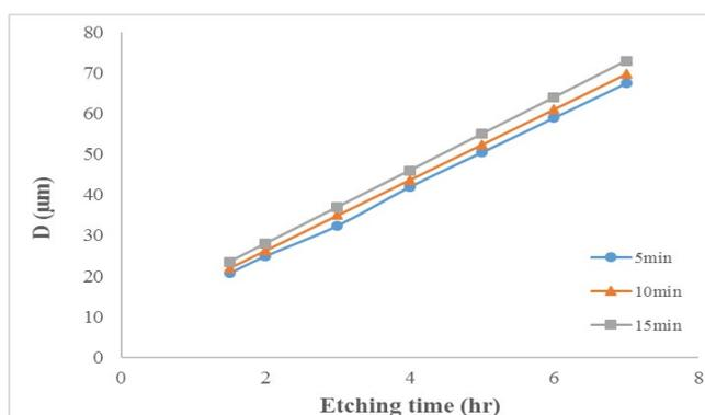
Figure 2: Alpha tracks diameter vs. etching time exposed to He-Ne laser beam at (5 mW) power etched in 6.25 N NaOH at  $60^\circ\text{C}$
