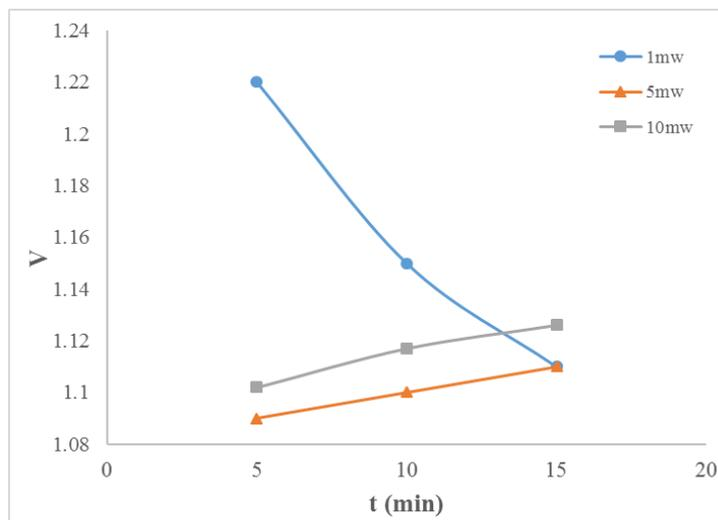
**Figure 13:** Etching rate ratio  $V$  vs. exposure time of He-Ne laser beam at different powers
