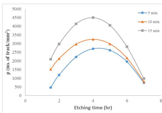
**Figure 6:** Alpha tracks densities vs. etching time exposed to He-Ne laser beam at power (10 mW) at different times etched in 6.25 N NaOH at 60°C
