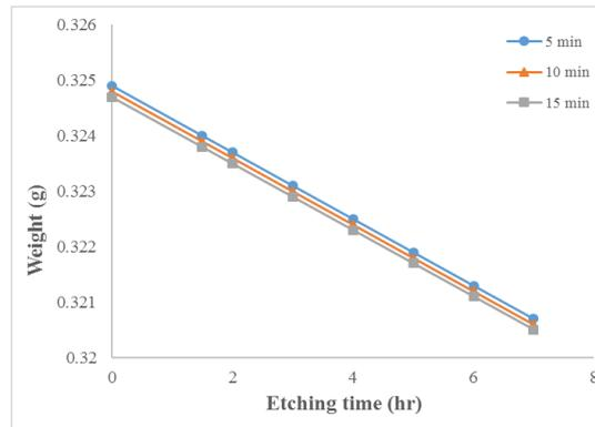
**Figure 7:** Weight of CR-39 detector vs. etching time at different exposed times to He-Ne laser beam at (1 mW)
