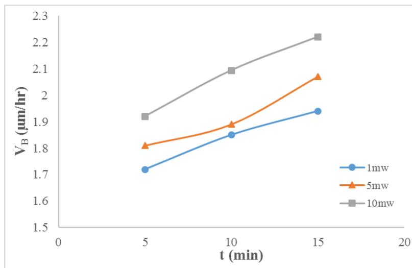
**Figure 11:** Bulk etch rate  $V_B$  vs. exposure time of He-Ne laser beam at different powers
