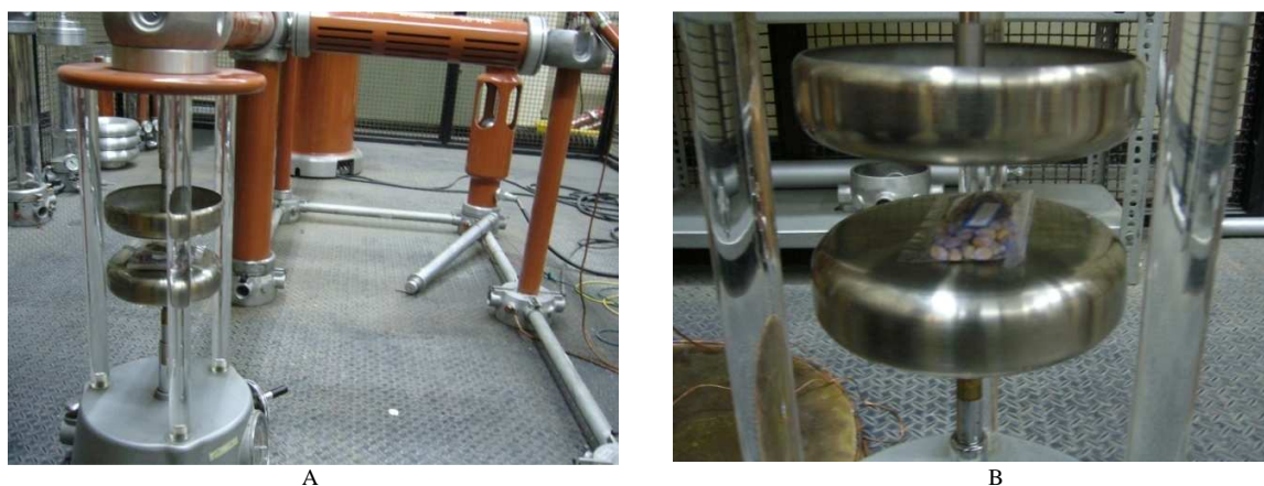
Fig. 1. Overall view of the electric field generator (A); Exposing maize seeds to electric field (B).
