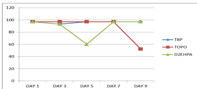
Figure 1: A plot of E% against day for the extraction of vanadium (V) from 6 Molar Hydrochloric acid with Tri butyl phosphate (TBP), Tri octyl phosphine oxide (TOPO), Bis-2-(ethylhexyl) phosphoric acid (D2EHPA).
