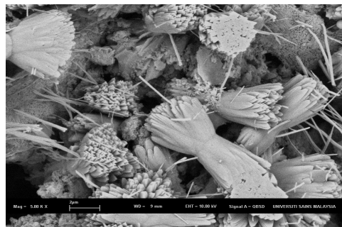
Figure 5. Transformation of complex particle by reaction of fly ash in hydration process
