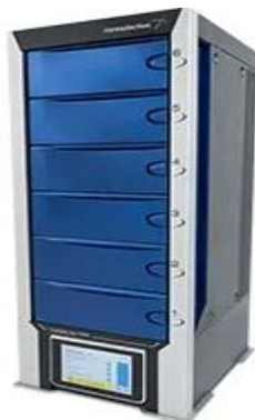
Picture 2: Formulation Turbiscan Tower [20]
