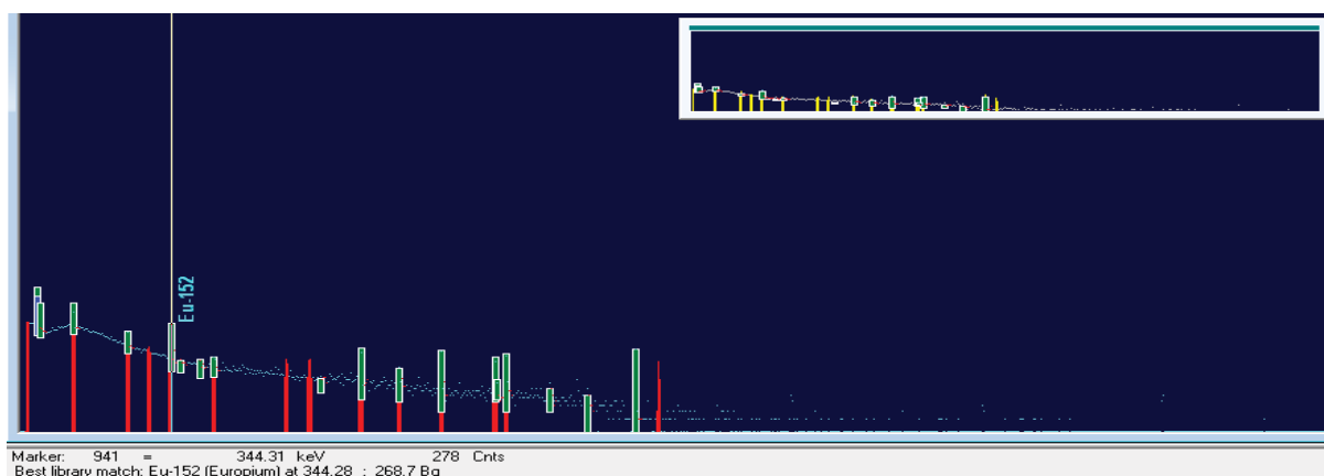
Figure 1: Represented the spectral analysis for soil contaminated with radionuclide Eu-152 (344) keV putted at drums (standard sample)
