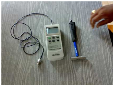
Fig. 3 Impactor and vibration meter
