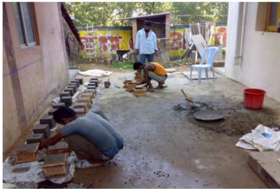
Fig. 1 Preparation of cubes
