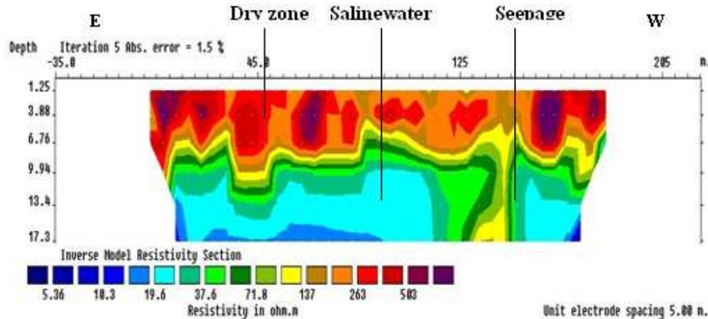
Fig.5 2D electrical resistivity imaging pseudosection along profile 2 depicts the seepage zone around the embankment of freshwater storage reservoir.
