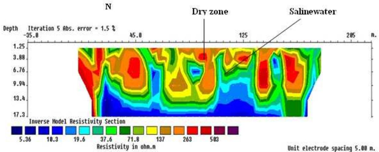
**Fig. 2** 2D electrical resistivity imaging pseudosection along profile 1 depicts the seepage zone around the embankment of freshwater storage reservoir.
