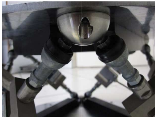
Fig. 2: The flexure joints used to connect the axes
