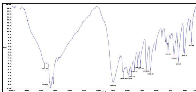
Fig. 5 FTIR Spectrum of Sr: BaC<sub>4</sub>H<sub>4</sub>O<sub>6</sub> 0.05M
