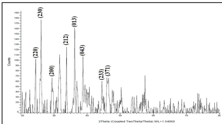
Fig. 2 XRD spectrum of Sr-doped Barium tartrate crystals
