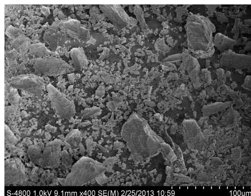
Fig. 3a-b. SEM picture of 0.05M Sr doped Barium tartarate crystals
