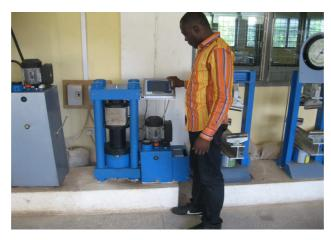
Figure 1. Compressive Strength Testing
