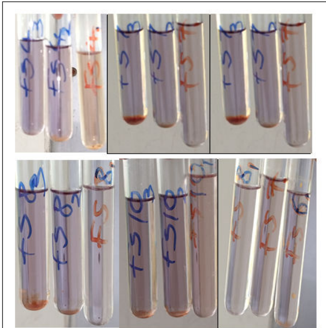
Figure 5: Treatment of Reactive Super Black dye waste water with PFS at varied pH.
