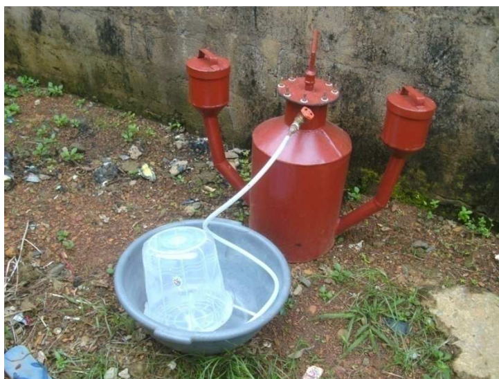
Figure 1: Experimental biogas plant set up
