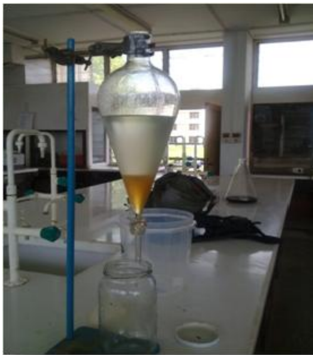
Plate 1. Separation of glycerin from coconut biodiesel
