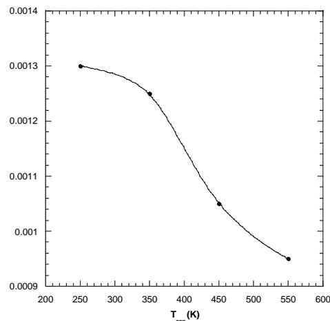
Fig.9 Variations of the resistivity  $\rho$  ( $\Omega \cdot \text{cm}$ ) with annealing temperature  $T_{ann}$  (K) for  $\text{Cd}_2\text{SnO}_4$  thin film of thickness 300 nm at room temperature.
