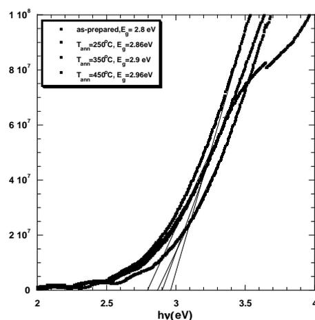
Fig.5 Plots of  $(\alpha h\nu)^{1/2}$  vs.  $h\nu$  for  $\text{Cd}_2\text{SnO}_4$  thin films, as-prepared and annealed at 250, 350, 450 °C for 2 hr.
