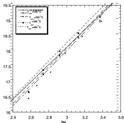
Fig 7  $\text{Ln } (\alpha) - h\nu$  relations for as-prepared and annealed  $\text{Cd}_2\text{SnO}_4$  thin films (300 nm thick) at different temperatures
