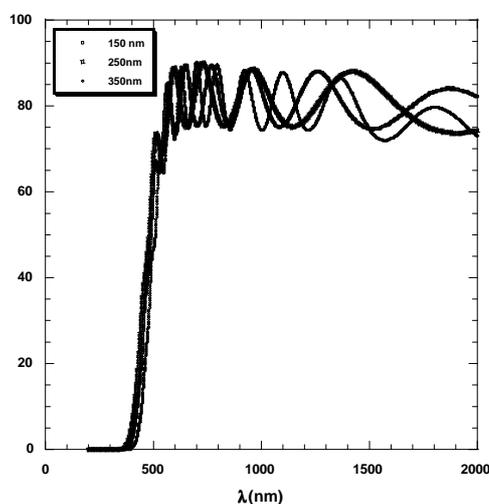
Fig.3 Variation of T% with  $\lambda$ (nm) for  $\text{Cd}_2\text{SnO}_4$  thin films of different thicknesses at room temperature.
