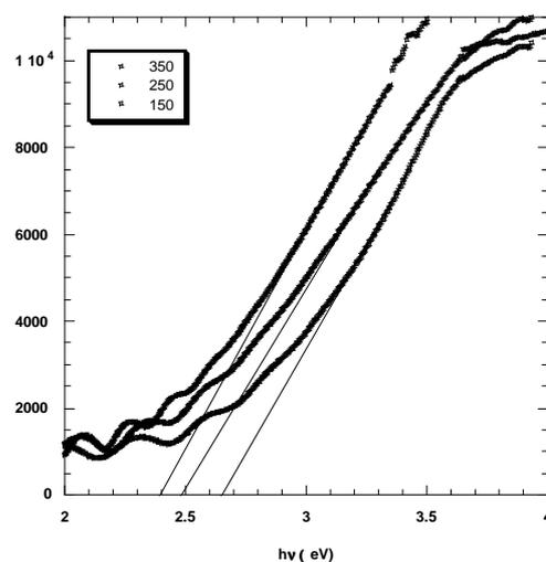
Fig. 6 plot of  $(\alpha h\nu)^{1/2}$  vs.  $(h\nu)$  for as-deposited  $\text{Cd}_2\text{SnO}_4$  thin films of different thicknesses
