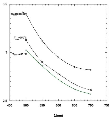
Fig.8 Variations of the refractive index  $n$  with the incident wavelength  $\lambda$  for as-deposited and annealed  $\text{Cd}_2\text{SnO}_4$  thin films of thickness 300 nm at different annealing temperatures for 20 mins.
