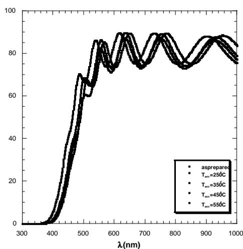
Fig.4 Variations of transmittance T% with wave length  $\lambda$ (nm) for as-prepared and annealed  $\text{Cd}_2\text{SnO}_4$  thin films at different temperatures.
