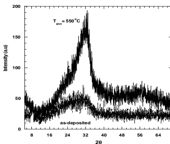
Fig. 1 X-ray diffraction of  $\text{Cd}_2\text{SnO}_4$  as-deposited and annealed thin films (350 nm thick) at 550 °c for 2 hrs.
