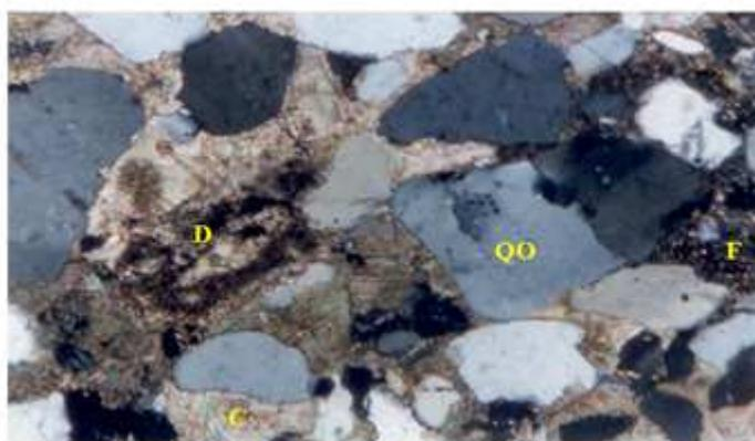
Fig. 8 Thin section photomicrograph exhibits middle to late diagenetic stages
