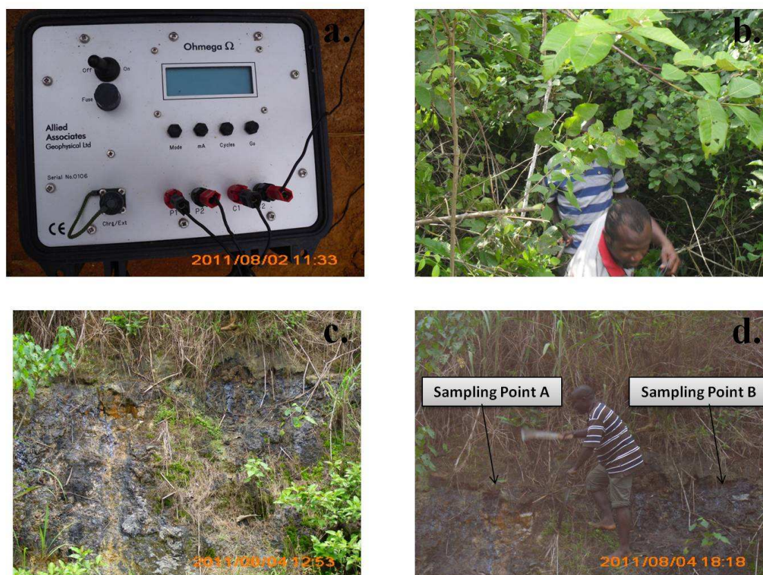
Fig 2: (a) The Ohmter Resistivity Meter used for the resistivity survey (b) Reeling of the Cables through the thick vegetation above the Seepage (c) The Bitumen Seepage, associated with is water running down the hill (d) Sample collection point for the lithofacies description
