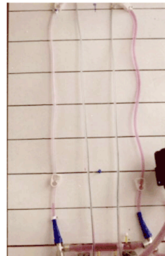
Figure 10. shows a circulatory model incorporating the G-C apparatus with manometers measuring PP, CP at points 1 and 7 and DP. Note that CP is lower than DP.
