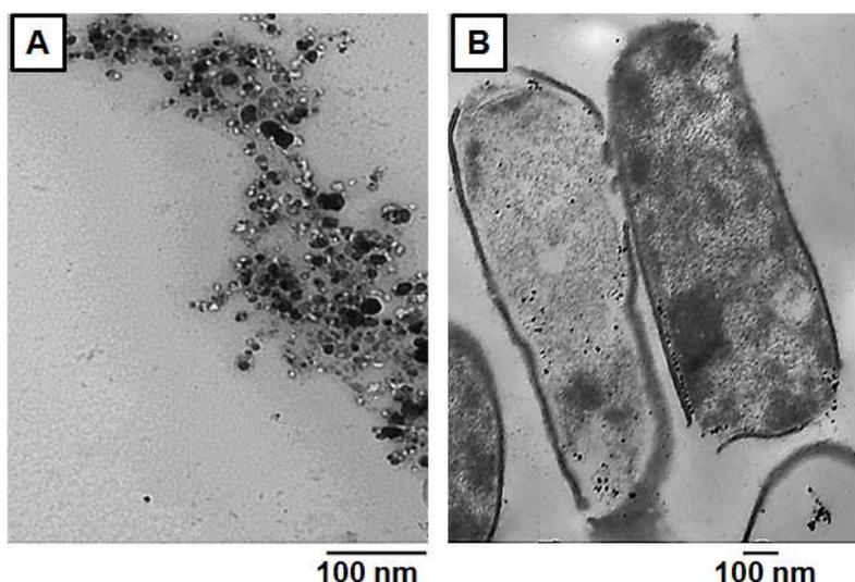
Figure 4: Transmission electron microscope image of Ag-NPs in culture broth (A), cross sections of strain 39M grown in 3.5 mM AgNO<sub>3</sub> (B)
