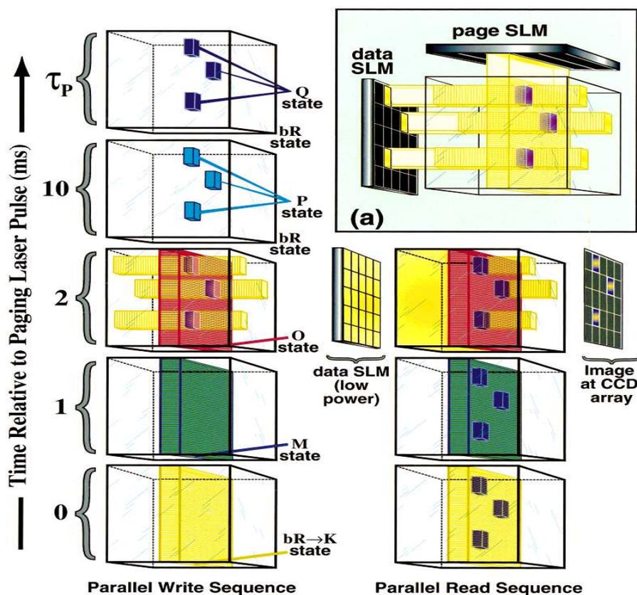
Fig. 6. Parallel write sequence (left) and parallel read sequence (right) for the hypothetical storage and retrieval of three bits of data in a page of memory using the branched-photocycle architecture.
