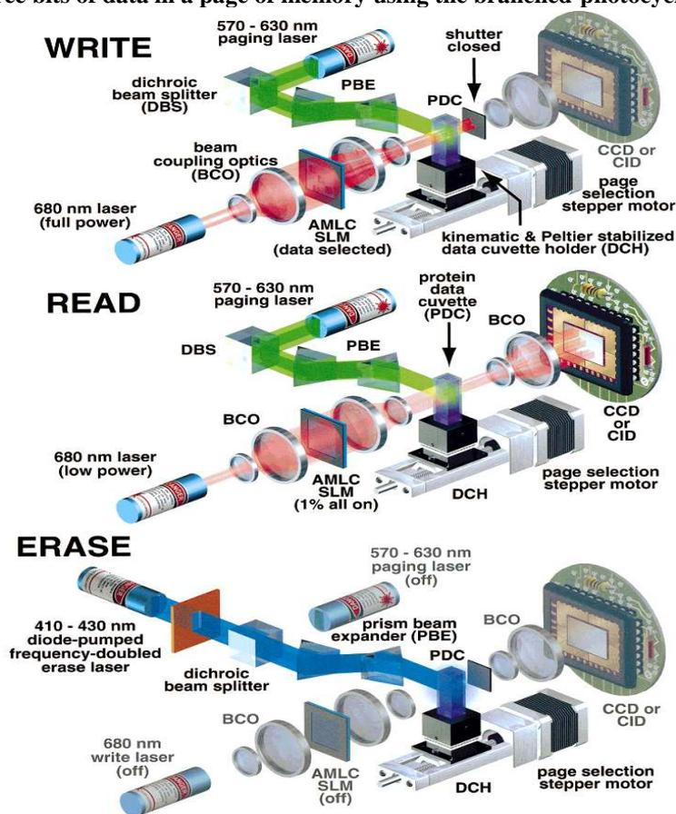
Fig. 7. Read, write, and erase processes based on a level I prototype design.
