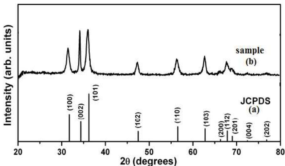
Figure. 1. XRD patterns of ZnO nanoparticles. (a) Indicate standard XRD pattern and (b) indicate sample XRD pattern
