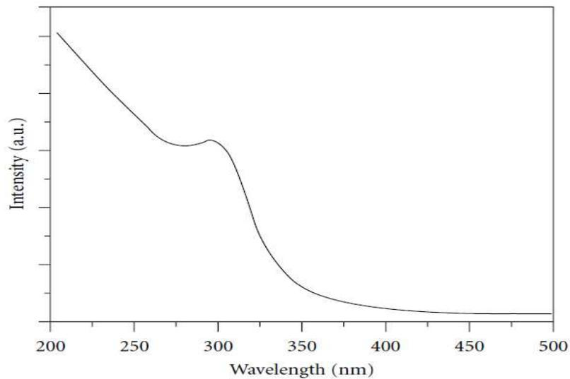
Figure 2. UV-Vis absorption spectra for ZnO nanoparticles
