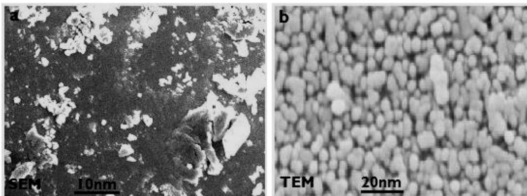
Figure 3. (a) SEM image and (b) TEM image, of ZnO NPs
