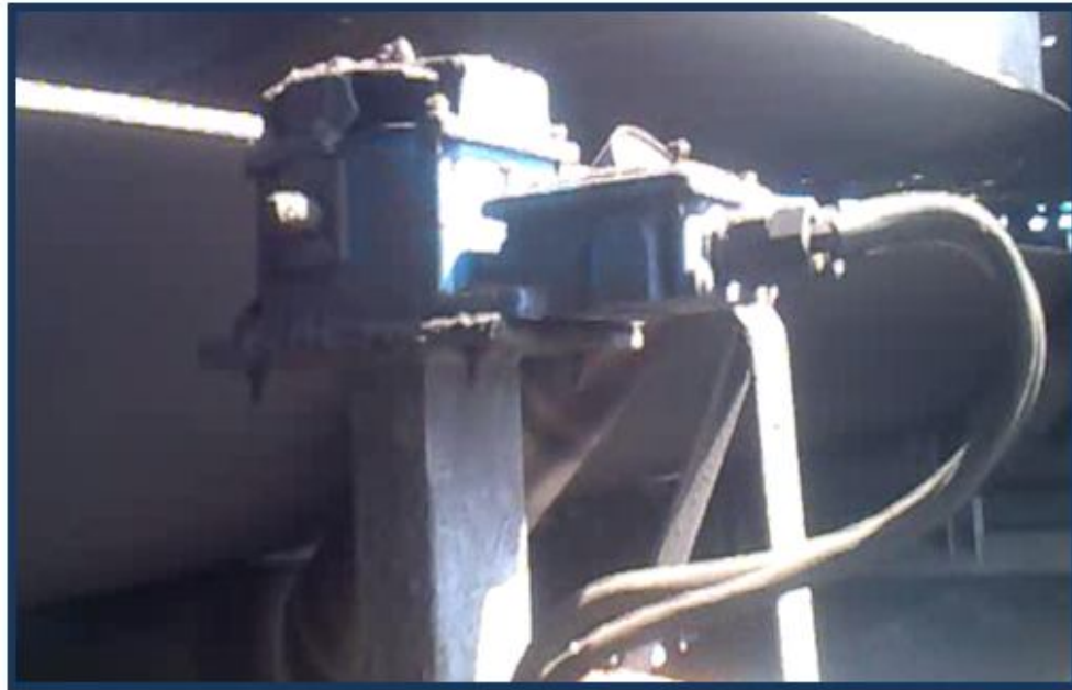
Fig.4. Image of Hydraulic control self-aligning-idler with displacement sensor
