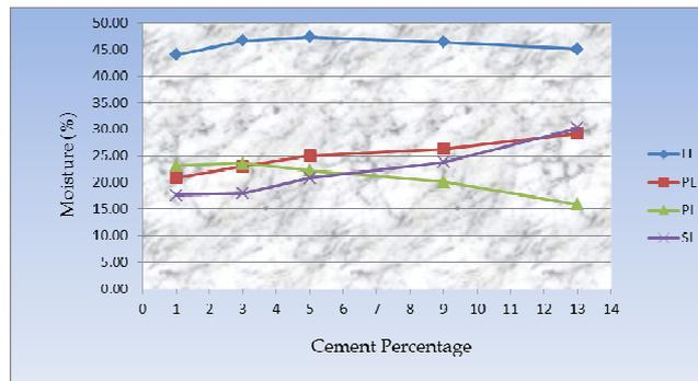
Figure 1. The effect of adding different percentages of cement on the plastic and shrinkage properties of the soil (PI = 20)
