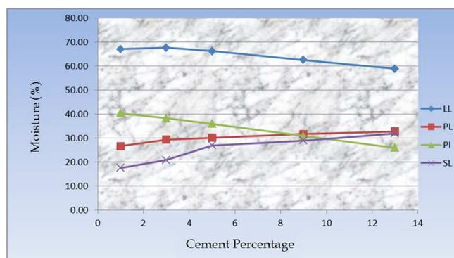
Figure 4. The effect of adding different percentages of cement on the plastic and shrinkage properties of the soil (PI = 40)
