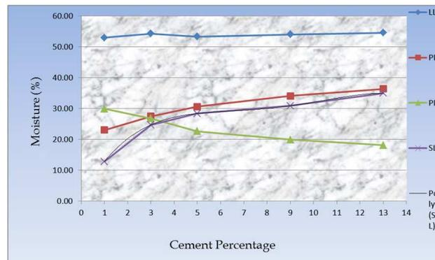
Figure 2. The effect of adding different percentages of cement on the plastic and shrinkage properties of the soil (PI = 30)
