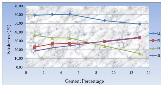
Figure 3. The effect of adding different percentages of cement on the plastic and shrinkage properties of the soil (PI = 35)
